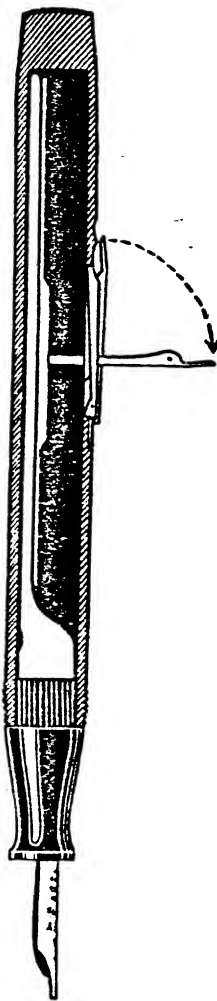
Note simple filling device and large interior area completely filled by sac
